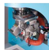
Easy-clean feed line damper valve
