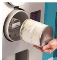
Front-of-system access for simple routine maintenance
